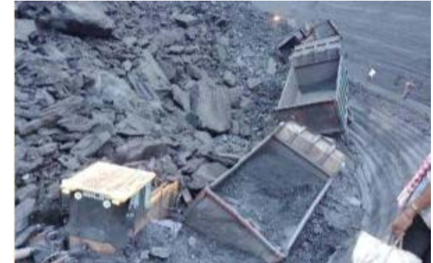
Failure of waste dumps
